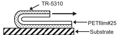
● 180 degree peeling strength for each temperature
